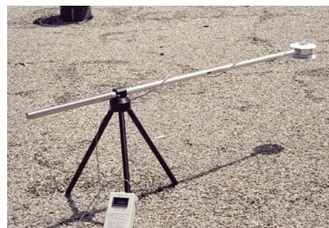
A mounted pyronometer measures albedo, the ratio of out-bound to in-bound solar radiation.
